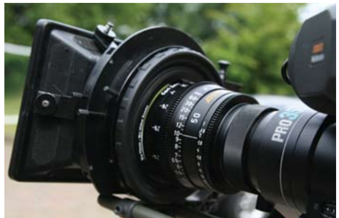
▲ Pro-35 Adapter with 35mm Ultra-Prime Lens. Lovely shallow depth of field – but challenging for the operator!
